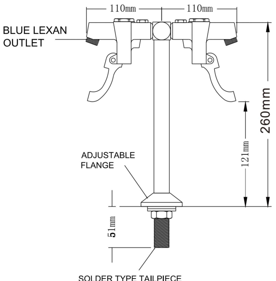
SOLDER TYPE TAILPIECE TO FIT1/4"O.D.TUBING. ALSO AVAILBLE TO FIT 3/8" & 1/2"O.D.TUBING.
